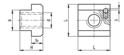
b -0.1 -0.3 = 22 d = M20 H = 28 h1 = 14 L = 35 I1 = 1.6 T-slot width DIN 650 = 22 Weight (g) = 155
